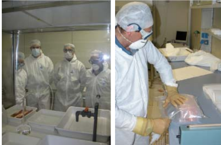
Figure 8: Chemical etching of Cu parts in clean room; on the right the sealing procedure in HP Nitrogen atmosphere of the etched materials is shown.
