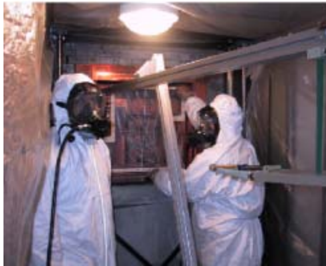
Figure 6: The dismounting of the detectors of the \simeq 100 kg set-up and the installation of the LIBRA detectors and PMTs' shield have been performed in HP Nitrogen atmosphere by using special masks connected to air bottles to avoid that the inner part of the Cu box, the detectors and the new PMTs' shield would be in contact with the environmental air, that is to reduce at most possible surfaces' contamination by environmental Radon.
