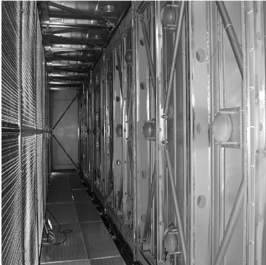
Figure 1: The 27 photomultipliers of one wall used for the detection of the scintillation lighth.
