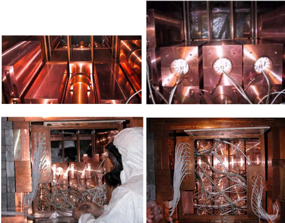
Figure 7: Left top picture: some detectors during installation; in the central and right upper detectors the new shaped Cu shield surrounding the light guides and the PMTs has not yet been applied, while it has in the other detectors nearby. Right top picture: in the 3 upper detectors the shaped Cu shield has been applied but the HV dividers are still visible. Left bottom picture: during the detectors installation. Right bottom picture: view at end of the detectors installation. All the used materials have been deeply selected for radiopurity (see for example the cables with teflon envelop).
