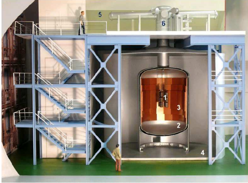
Figure 1: An artist’s view of the GERDA detector. The array of Ge detectors is not to scale. (1): the array of germanium detector string; (2): the stainless steel cryostat; (3): copper lining; (4): the water tank; (5): the clean room; (6): the lock. Plot from Ref. [1].
