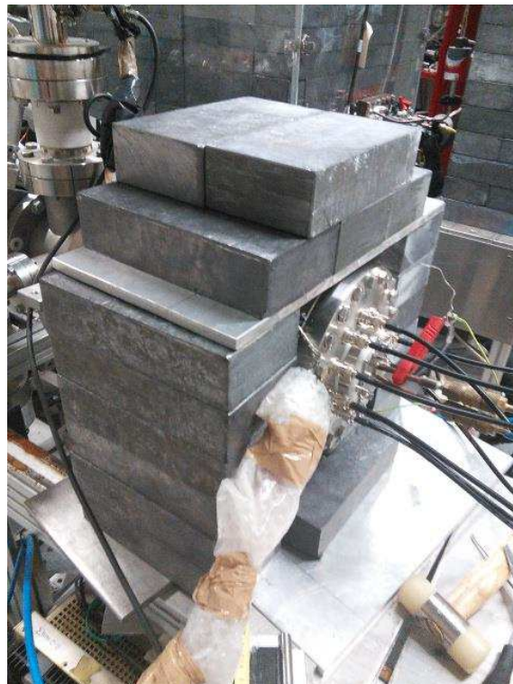
Figure 1: (top) A picture of the scattering chamber before mounting the detectors. The proton beam enters from the copper tube on the top. (bottom) The chamber mounted horizontally on the beamline and shielded with lead.
