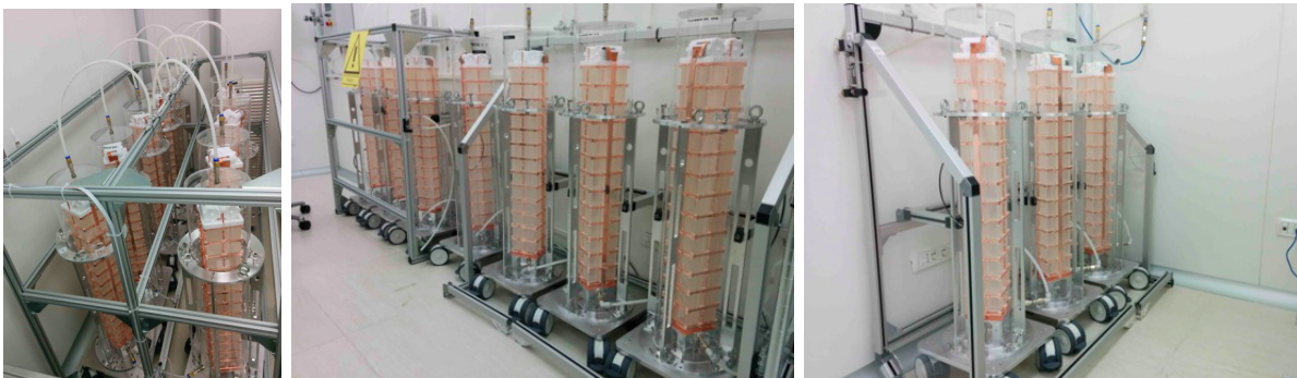
Figure 8: Part of the ready-to-mount detector towers in their storage inside the CUORE clean room.
