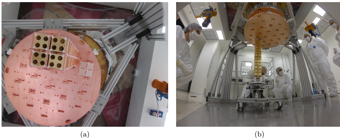
FIG. 11. (a) TSP fixed with the DIT, with mockup tower installed. (b) A moment during the mock-up tower installation, with the DIT installed and the DIC to position the tower.
