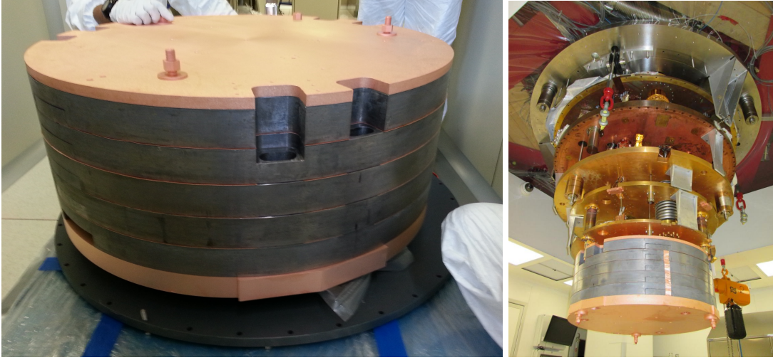
FIG. 2. Top lead shield assembly at LNGS (left) and after installation, suspended inside the CUORE cryostat (right).
