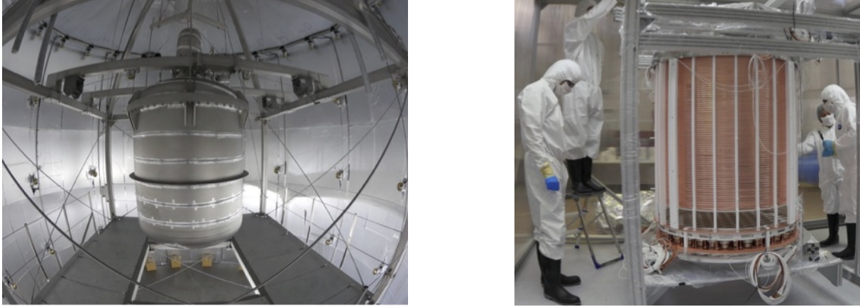
Figure 5: Left: XENON1T cryostat suspended by the support structure inside the water tank. Right: Assembled TPC in the cleanroom of Lab2.
