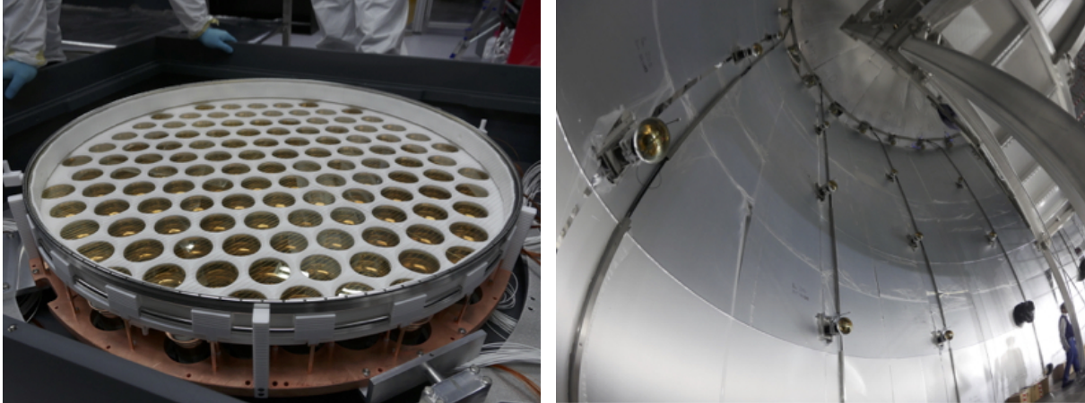
Figure 7: Left: Assembly of the Bottom PMT array with screening mesh and cathode. Right: Muon veto system with reflective foil (behind protective foil).
