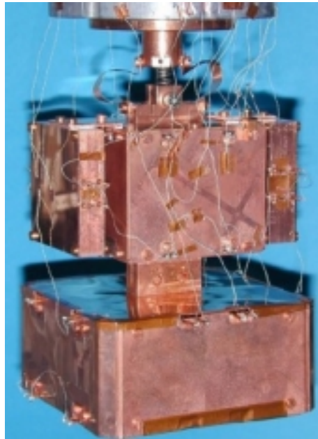
Figure 7: Two 4-crystal arrays are mounted simultaneously in Hall C test facility
