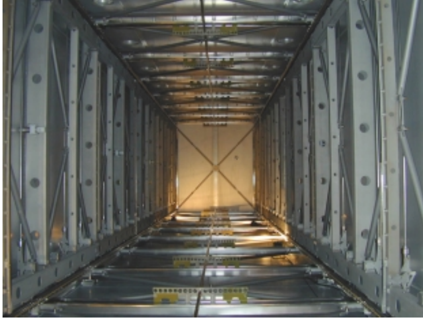
Figure 3: Picture of the whole internal detector sustaining structure inside the first half-cryostat.
