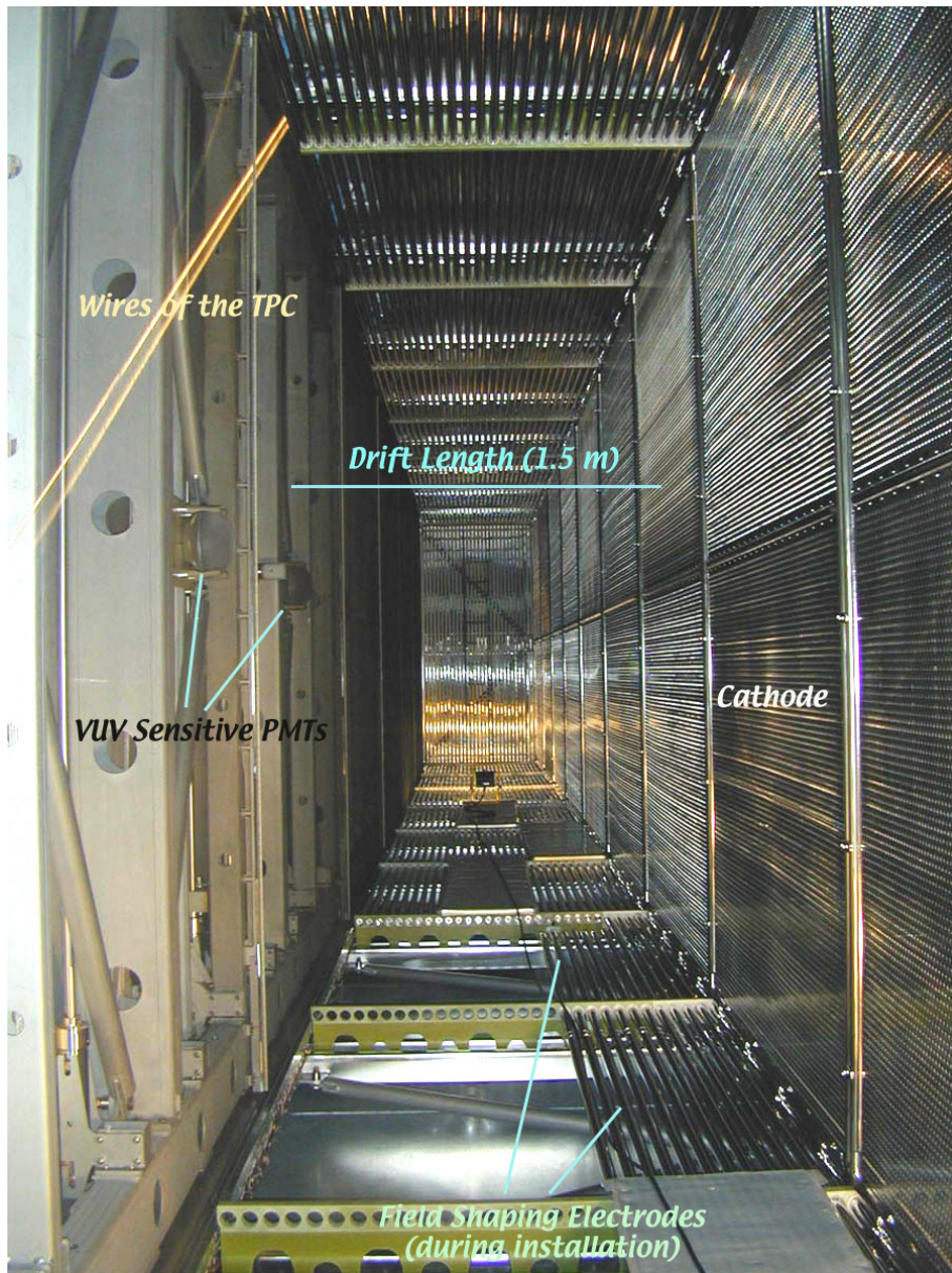
Figure 3: Picture of the inner detector layout inside the first half-module: the cathode (vertical plane on the right) divides the volume in two symmetric sectors ( chambers ). The picture refers to the left sector where wires and mechanical structure of the TPC and some photo-multipliers (PMTs) are visible.
