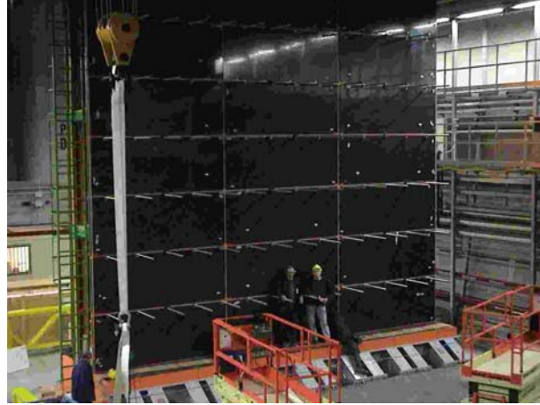
Figure 3: Installation of the first RPC plane in the OPERA spectrometer at LNGS
