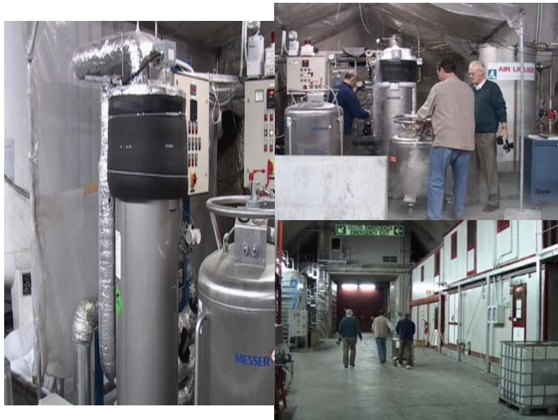
Figure 6: BOREXINO-GENIUS-TF nitrogen purification system in GRAN SASSO (left and upper right). The left part shows the absorber column (low temperature absorber - LTA) provided by the GENIUS-TF group. The nitrogen is transported by 200l vessels to the GENIUS-TF building (lower right).
