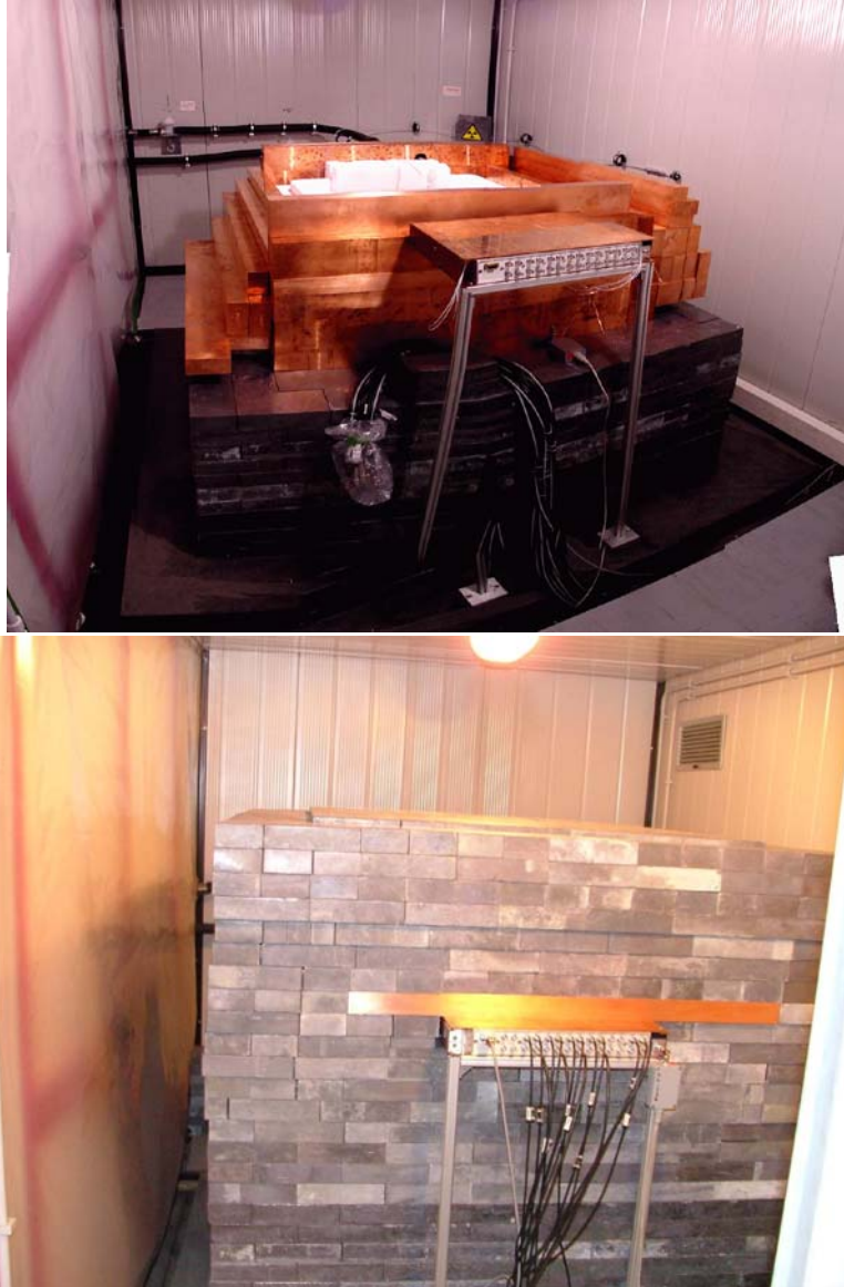
Figure 4: View of GENIUS-TF in the Gran Sasso Underground Laboratory in Italy. Left: The setup with detectors inside, but shielding only partly mounted. In front the preamplifier system. Status May 5, 2003. Right: The full shielding of GENIUS-TF, status December 2, 2003.
