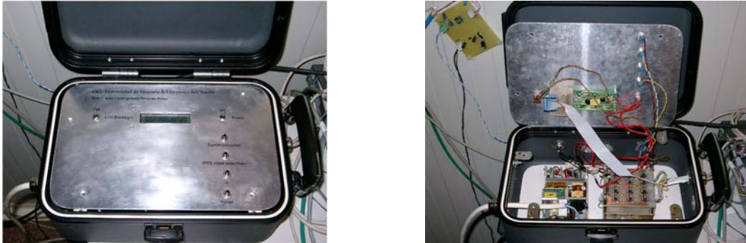
Figure 4: The Underground Array seismic stations acquire data simultaneously. The time synchronization is controlled by a Master Oscillator: it takes a 1 pps input signal from an atomic clock located in the labs and generates codified time signals which are send to the single stations in order to provide simultaneous data acquisition.
