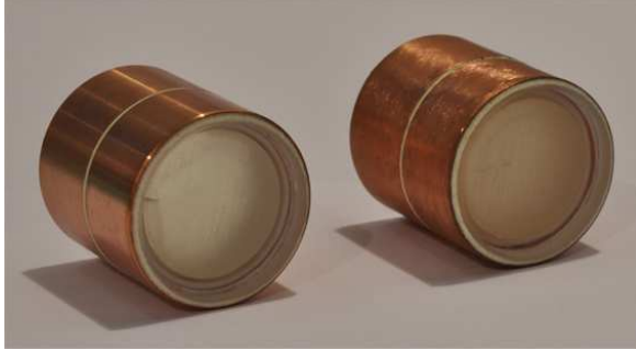
Figure 4: (Color online) Left: the enriched {}^7\text{Li}(\text{Eu}) crystal scintillators. Right: energy spectrum accumulated with the {}^7\text{Li}(\text{Eu}) sample No. 1 (red histogram) over 778 h by ultra-low background HPGe \gamma spectrometer. The background spectrum measured without sample over 3047 h (green histogram) is also shown. (Insert) Low energy part of the spectra. The energies of \gamma lines are in keV.
