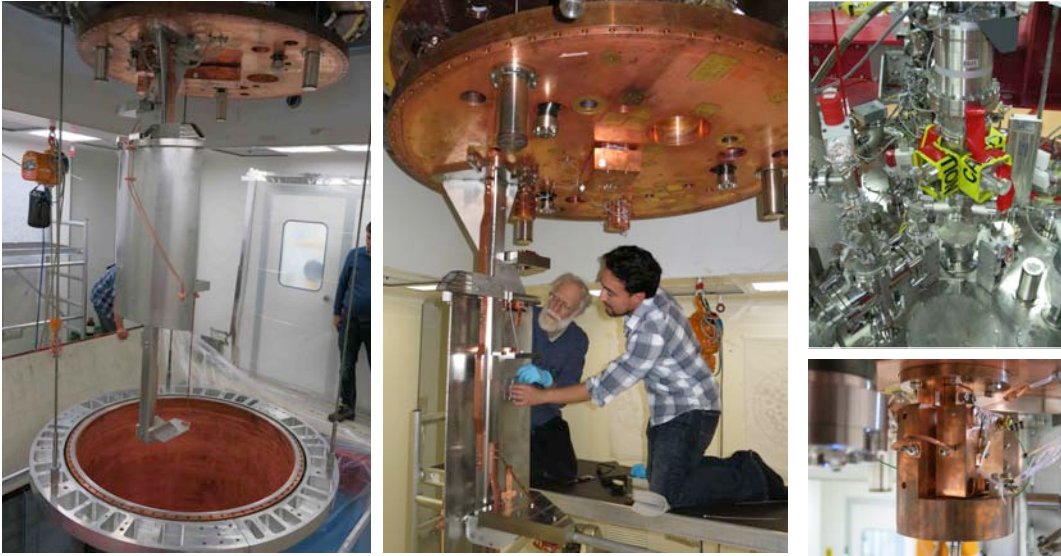
Figure 3: Cooldown test of the Detector Calibration System. Left and middle: Mockup of the internal cryostat structure and guide tube system. Right: Deployment system above 300 K (top) and mechanical source thermalization mechanism below 4 K (bottom).
