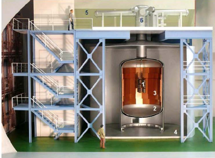
Figure 1: An artist’s view of the GERDA detector. The array of Ge detectors is not to scale. (1): the array of germanium detector string; (2): the stainless steel cryostat; (3): the radon shroud; (4): the water tank; (5): the clean room; (6): the insertion lock. Plot from Ref. [1].
