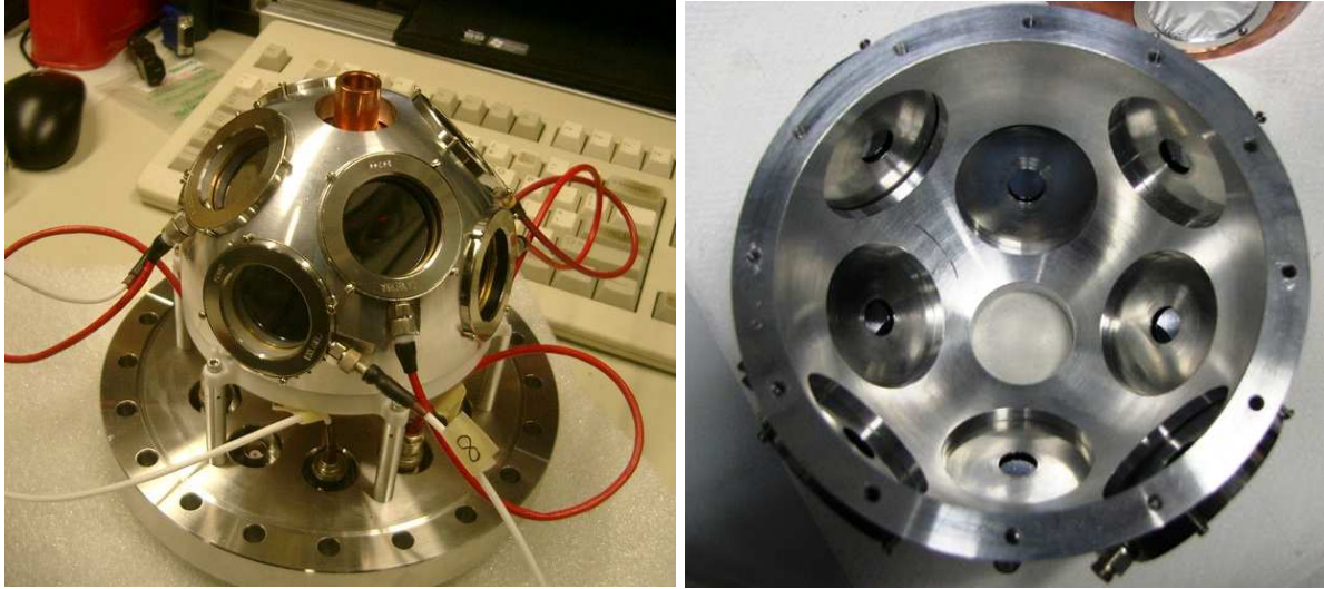
Figure 1: (Left) the scattering chamber with the silicon detector mounted. The proton beam enters from the copper tube on the top. (Right) the inside of the aluminium dome on which the detectors are mounted, showing 1 cm diameter collimators.
