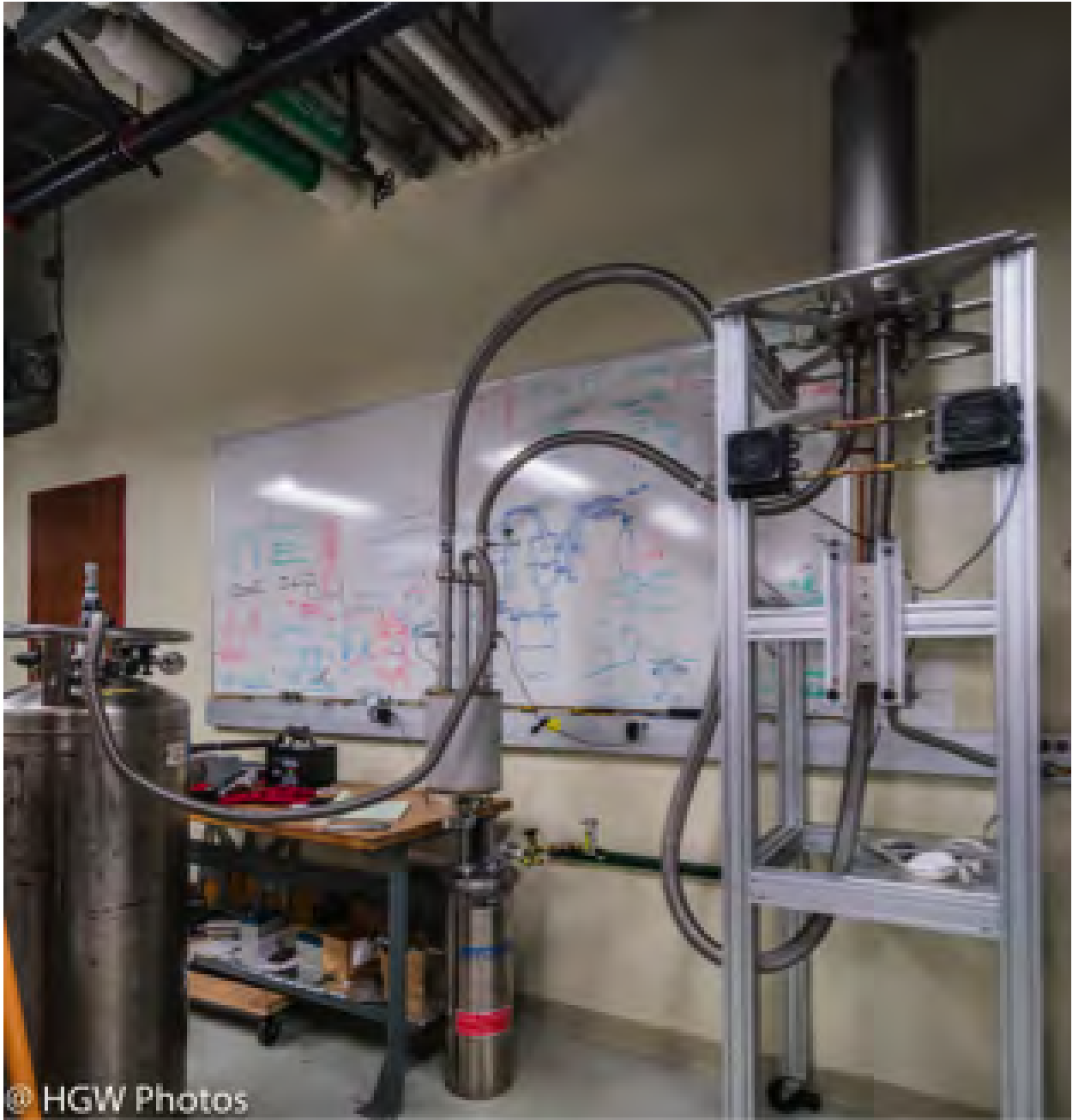
FIG. 7. DarkSide-Proto : laboratory test of the full scale condenser.
