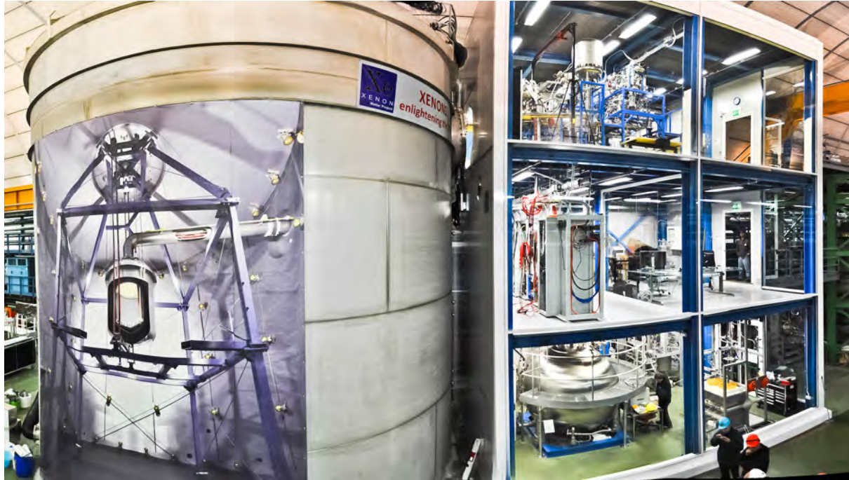
Figure 3: View of the XENON1T experiment in Hall B of the LNGS. The cryostat housing the dual-phase xenon TPC is hanging in the middle of the water tank. The service building with all equipment to support running the experiment, has three, fully packed, floors.
