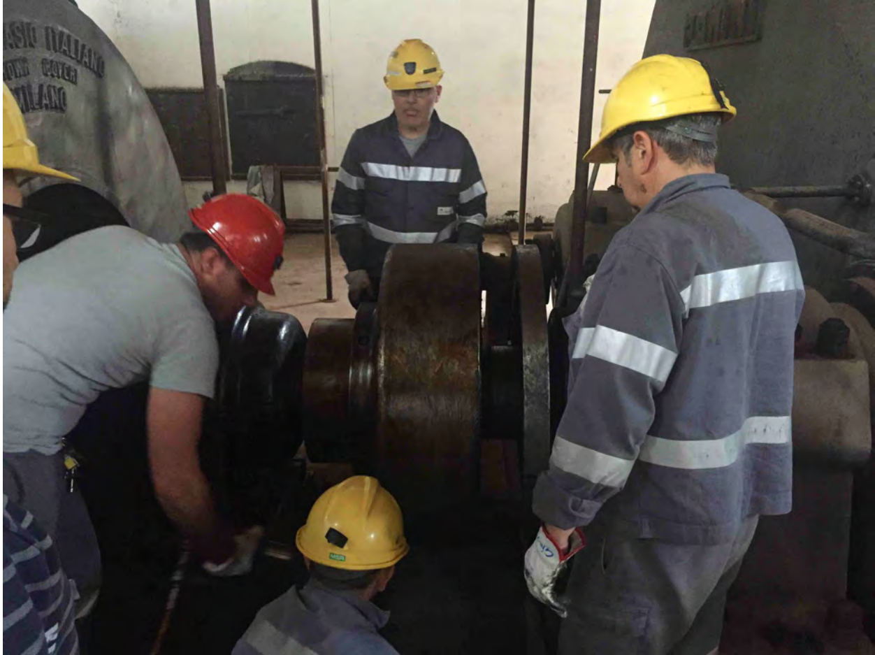
FIG. 12. Aria: first coupling of the motor to the Seruci winze wheel, Summer 2016.
