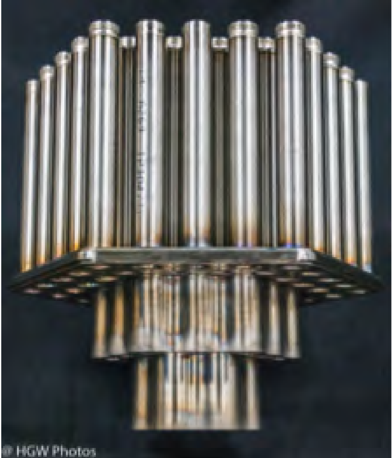
FIG. 6. DarkSide-Proto : the condenser heat exchanger.
