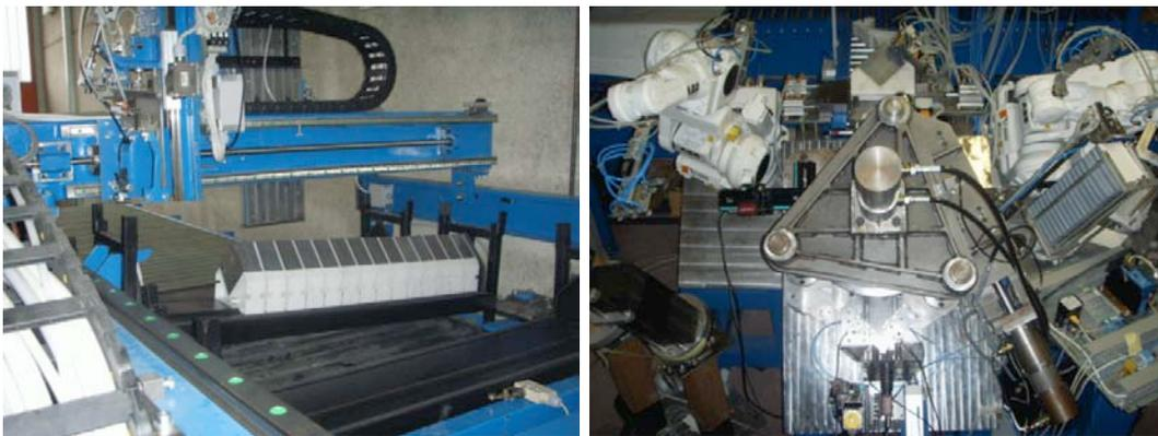
Figure 7: The automatic system to handle lead transportation boxes.
