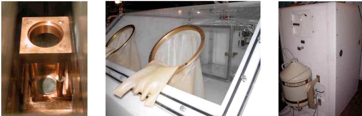
Figure 11: New shield and Marinelli system of the DAMA/Ge set-up.
