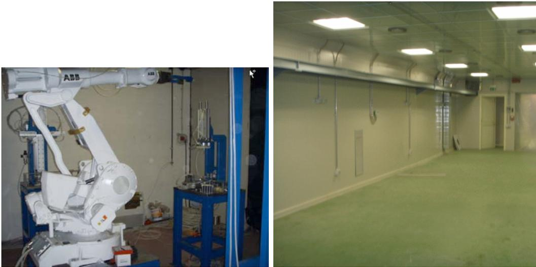
Figure 9: The wrapping station of the brick with Al tape.
