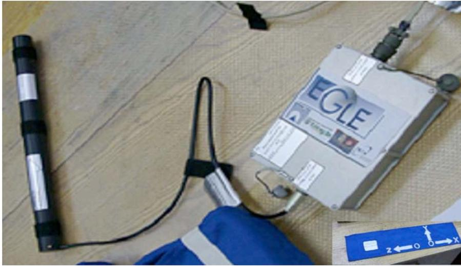
Figure 1: Egle box and Egle magnetometer head
