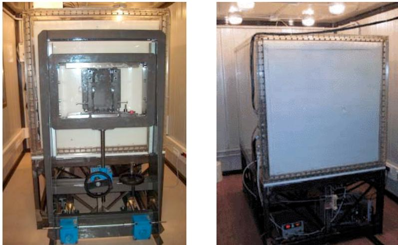
Figure 8: Shield of the DAMA/R&D set-up and the automatic system to close it.
