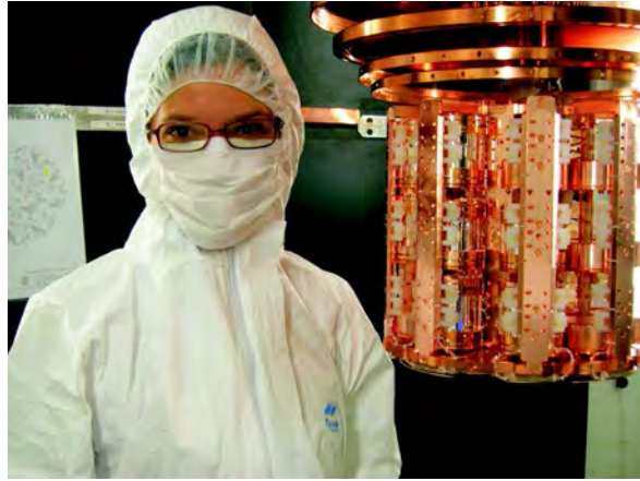
Figure 8: Installation of the first 9 detector modules in CRESST II.
