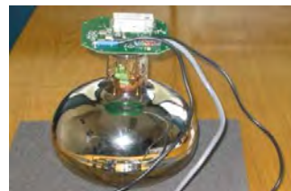
Figure 1: The XP1805/D1 photomultiplier and the dedicated two outputs, last dynode amplified base.
