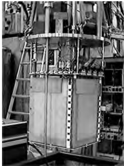
Figure 2: The 50 liters Liquid Argon Time Projection Chamber.
