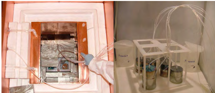
Figure 1: Left - View from the top on the GENIUS-TF-II setup during installation in October 2004. Right - The six contacted naked Ge detectors.
