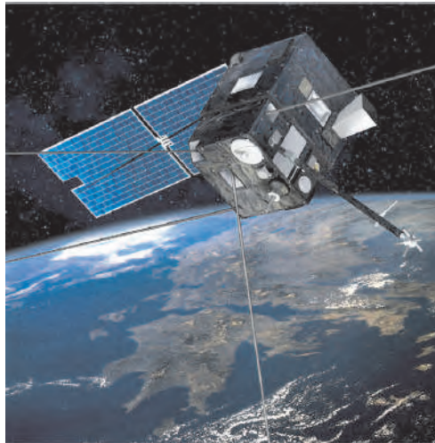
Figure 2: Picture of the Demeter satellite in flight with its deployed booms and sensors.
