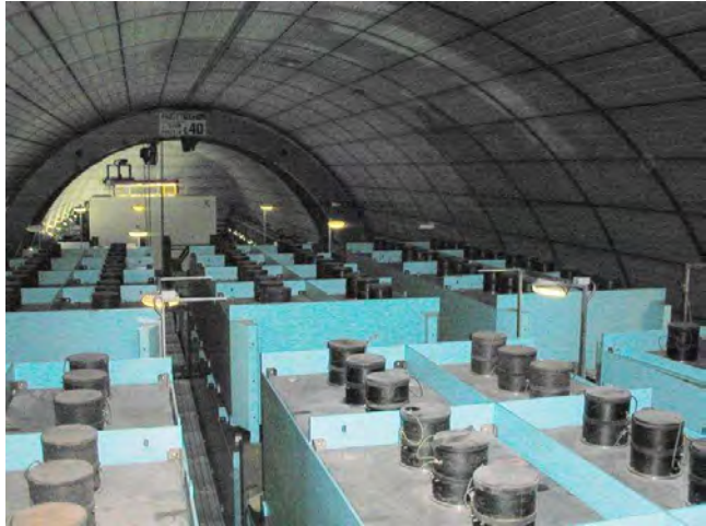
Figure 2: Top view of the LVD detector in the hall A of the Gran Sasso National Laboratory, INFN.
