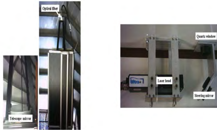
Figure 3: The present Raman Lidar telescope on the top of the Lidar shelter in Los Leones and the new laser configuration inside the shelter, firing to the steering mirror.
