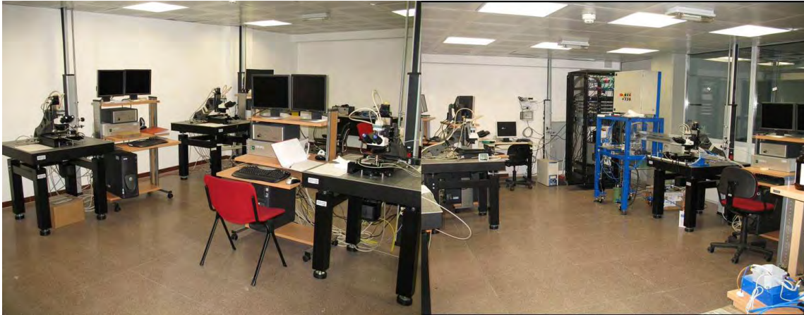
Figure 3: The OPERA Scanning Station in the outside Laboratory. During 2006 the installation of 6 microscopes with computer control, has been completed. The microscopes will be mainly used for the scanning of the changeable sheets to look for tracks of charged particles validating the occurrence of a neutrino interaction in the corresponding brick.
