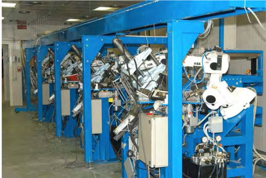
Figure 4: The piling/pressing station of the Brick Assembly Machine (BAM) in the underground laboratory. It consists of 6 anthropomorphic robots which have to assemble the bricks alternating emulsion and PB sheets. The final brick production rate should reach the value of 1000 bricks/day.
