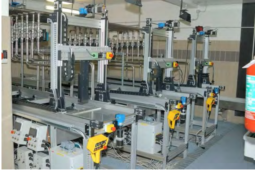
Figure 5: Partial view of the emulsion development laboratory realized during 2006 in the new LAB1 building. Three of six computer controlled chains of development are shown in the picture and are already working, the other three are in completion phase.
