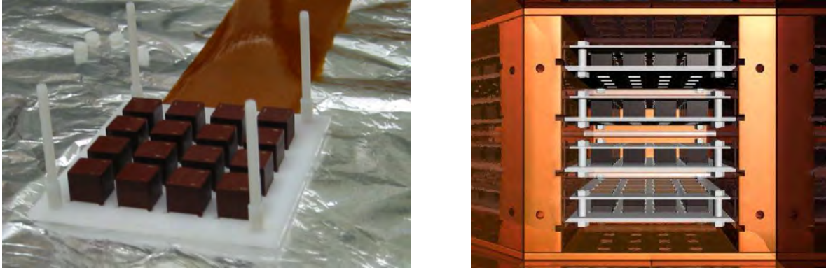
Figure 2: A photograph of the first layer of the 64-crystal proto-type (left) and an engineering model of the whole array in the copper mounting structure (right).
