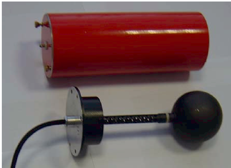
Figure 9: Electric field probe
