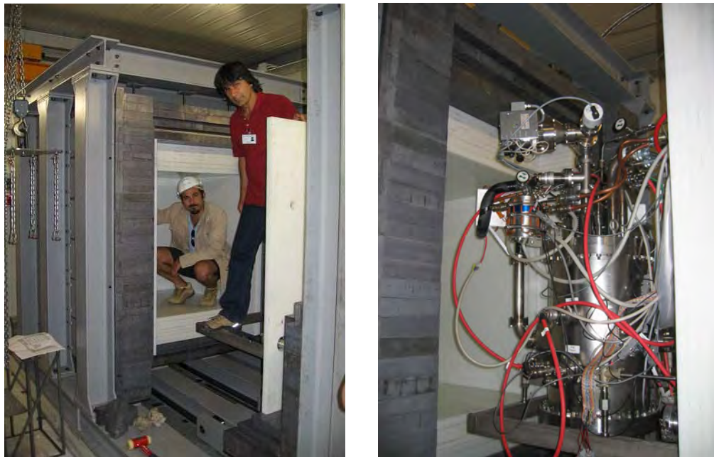
Figure 5: The XENON10 lead/poly shield, before (left) and after (right) the detector installation.
