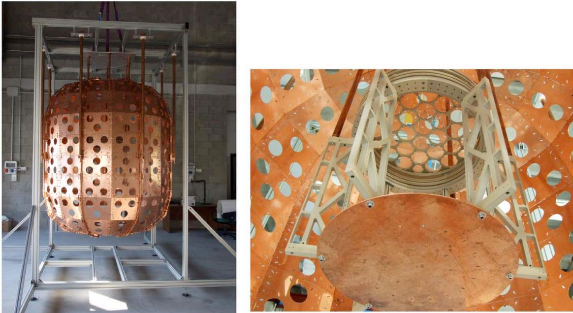
Figure 4: *View of the WArP -100 active Veto structure during the assembly test.*
