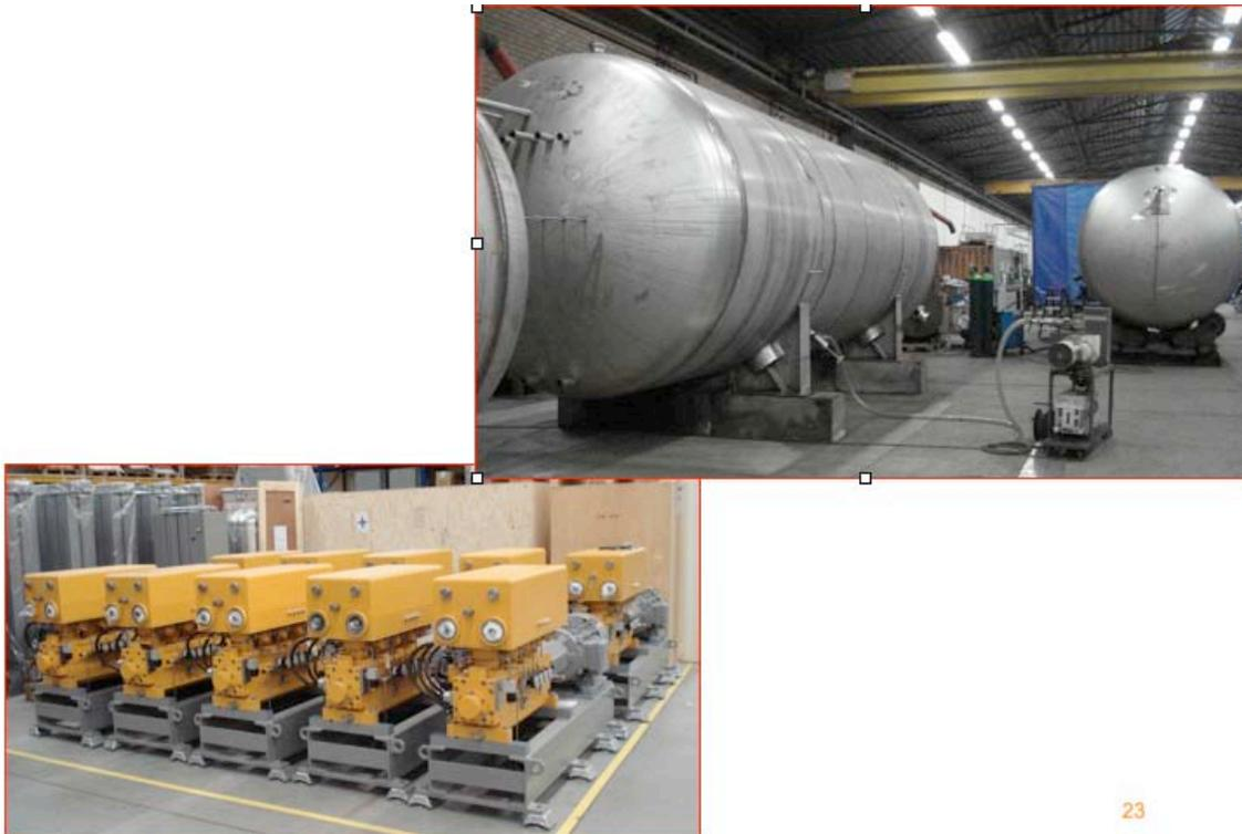
Figure 12: *Components of the Nitrogen re-liquefier system.*
