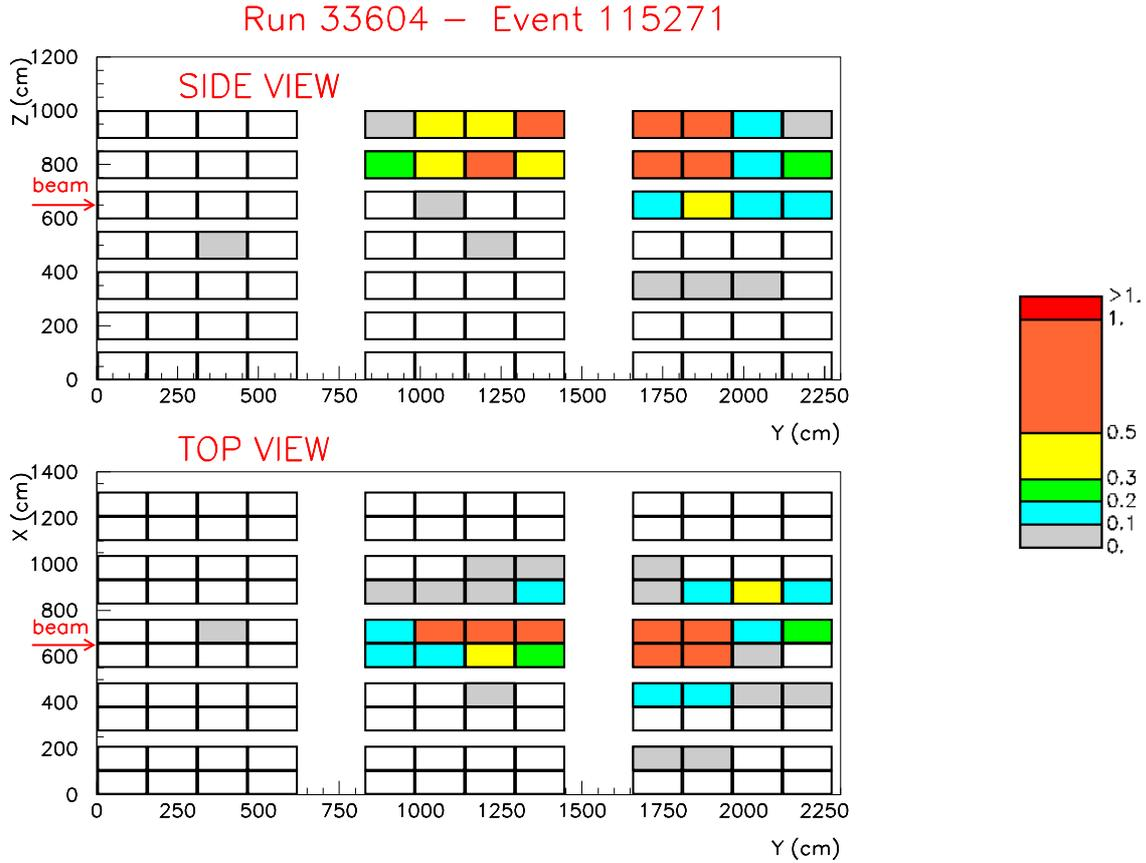
Figure 13: Display of a CNGS events: neutrino interaction inside the LVD detector. The colours represent the amount of energy released in the scintillation counters; the legenda is expressed in GeV.
