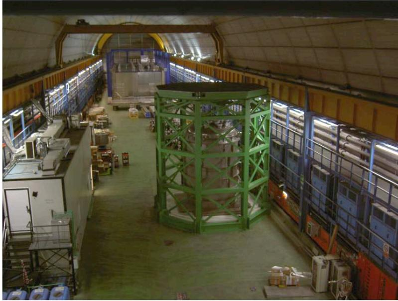
Figure 6: *Picture of the WArP -100 experimental site in HALL-B (underground LNGS). Visible the cryostat in its final position, inside the external shield sustaining structure.*
