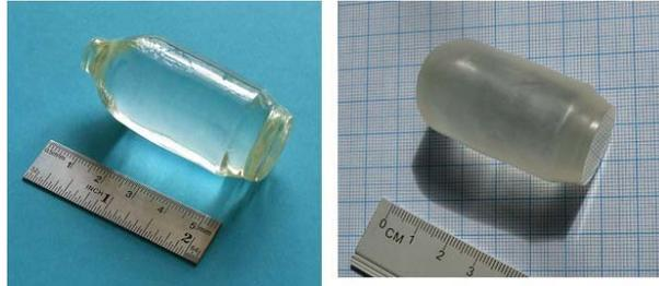
Figure 5: Boule of  $^{106}\text{CdWO}_4$  single crystal grown by the low-thermal-gradient Czochralski process (left; the scale is in centimeters and inches). Scintillation element  $^{106}\text{CdWO}_4$  with mass of 215.8 g produced from the boule (right; the scale is in centimeters). The side surface of the scintillation element was made diffuse with the help of fine-grain polishing paper to improve the uniformity of the scintillation light collection.
