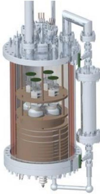
Figure 3: *Layout of the vessel and inner 2.3 lt chamber. In the present test the LAr level inside the vessel is above the PMT bases (i.e. the detector is operated in single liquid-phase).*
