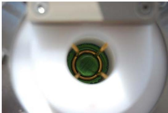
Figure 10: Tantalum Oxide target: brilliant color due to the oxide/metal interface interference were observed. Each color is related to a different thickness.
