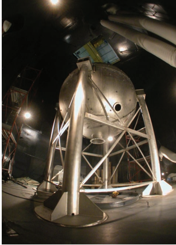
Figure 2: A photograph of the inside of the CTF water tank showing the Stainless Steel Sphere which contains the scintillation veto
