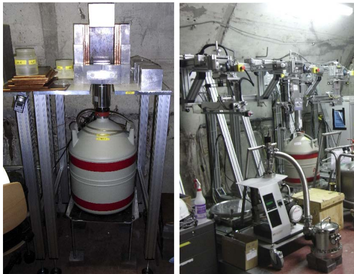
Figure 6: Setups used for the characterization measurements. Left: Setup for static source measurements. Right: Automated scanning tables.
