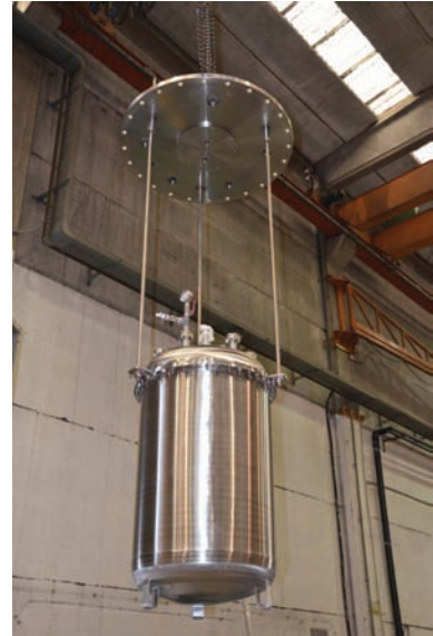
Figure 4: A photograph of the DarkSide50 cryostat hanging from a flange similar to the flange on top of the CTF
