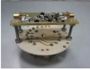
Figure 5: A picture of the cold preamp board mounted on the PMT base
