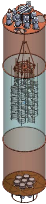
Figure 8: Schematic of the hybrid design for the LAr scintillation veto. The central cylinder (in gray) is composed of scintillating fibers.
