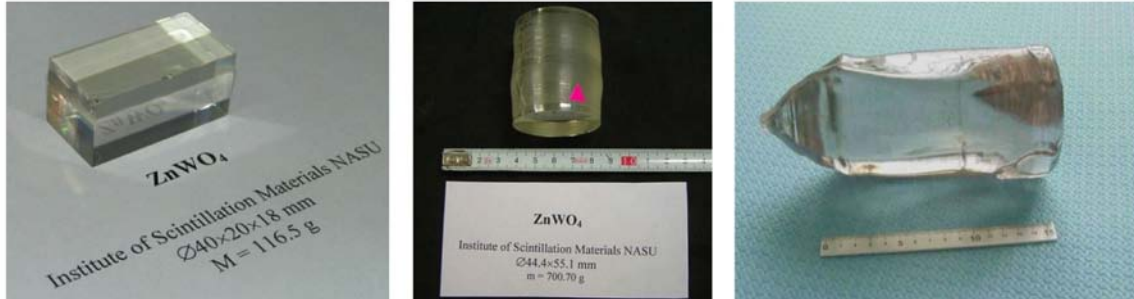
Figure 8: Three of the \text{ZnWO}_4 crystal scintillators recently developed [43]. Two \text{ZnWO}_4 samples (left and middle pictures) have been grown in the Institute of Scintillation Materials (Kharkiv, Ukraine). The crystal in the right picture has been produced in the Nikolaev Institute of Inorganic Chemistry (Novosibirsk, Russia); it is \simeq 8 cm in diameter and \simeq 15 cm length of cylindrical part.
