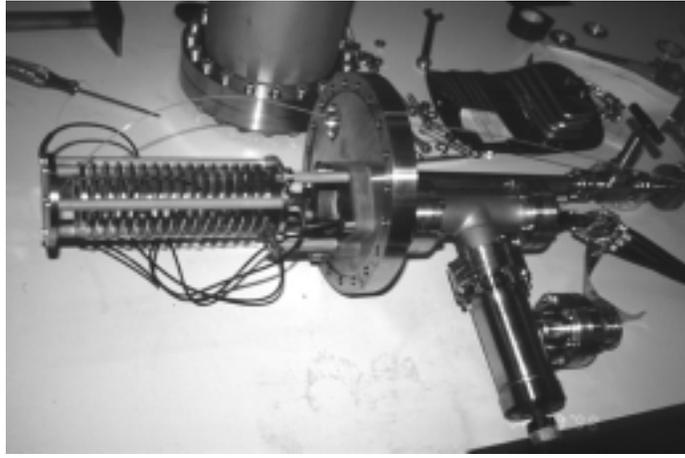
Figure 10: The *LAr* purity monitor built at LNGS
