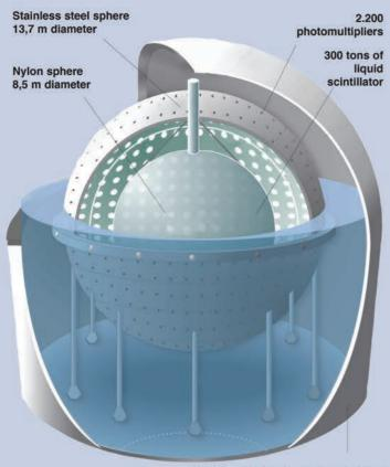
Stainless steel water tank with 2.400 tons of ultrapure water
